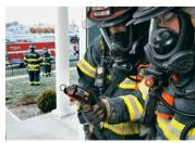
Special monitors are needed to detect the presence of carbon monoxide in the environment
