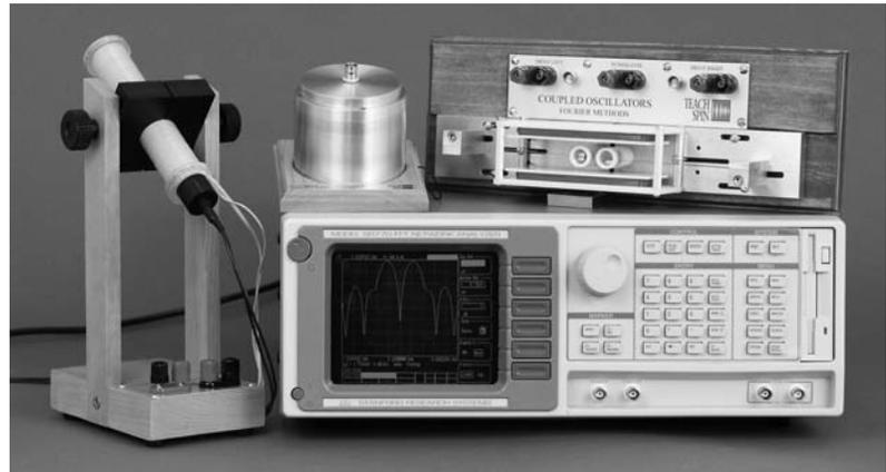
voltage. Fig. 2 shows the 770's view of the spectrum of this VCO's output, when it is set for a 50-kHz center frequency, with a 1-kHz modulation frequency. This spectrum shows the existence of sidebands, and the frequency 'real estate' required by a modulated signal. It also shows that Volt-level signals can be detected standing > 90 dB above the noise floor of the instrument.
