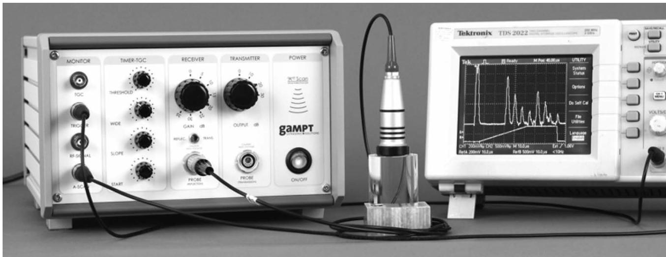
**Fig. 6: The echoscope set-up**
