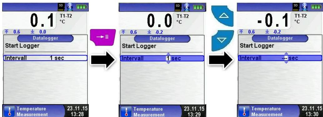
Then confirm with the “Enter” button and set the second number. Again confirm with “Enter” button and finally set the third number. Confirm the number with “Enter” button.
