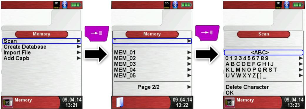
Select with the arrow keys the row with the desired character. Open the row with the „enter key“ and select the desired character using the arrow keys. Select letter by letter in this way:
