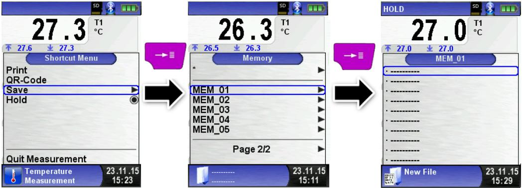
The file name and the storage location is shown in the lower bar. In this example: Storage folder: MEMORY/0000 and file name 0000\_00.txt:
