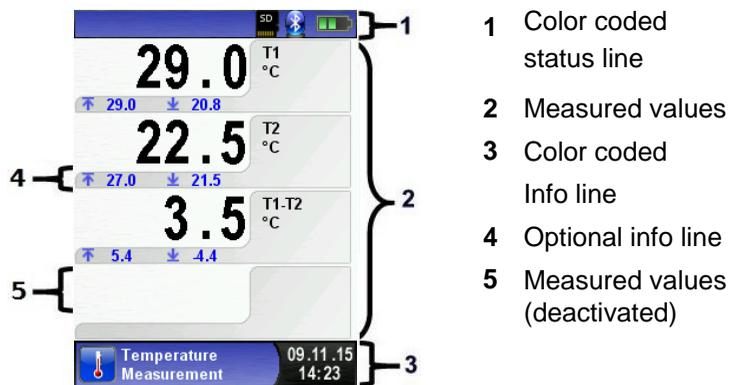
Fig. 6: Display showing measuring program (example: Temperature measurement)
