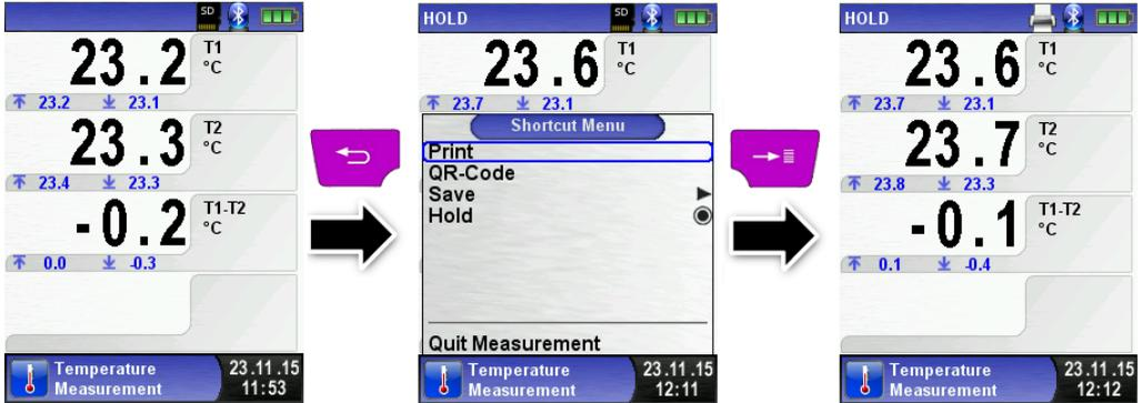
As soon as the print command is chosen, the record is printed parallel to the measuring task (→ multitasking function), i.e. the measurement mode remains active.
