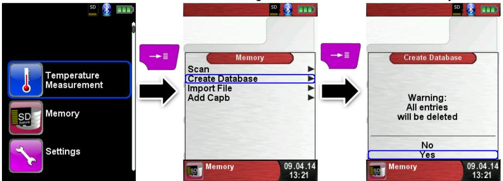
With this procedure a file named DATABASE.CSV will be generated on the MicroSD card. This file will show the database entries of the TMD9. This process needs a few seconds.
