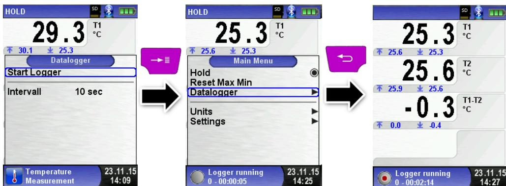
Stop the Datalogger with the “Enter” button on “Stop Logger”.
