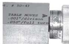
RIVETER table advancing knob detail
