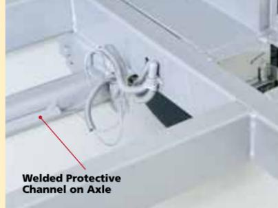
Welded Protective Channel on Axle
