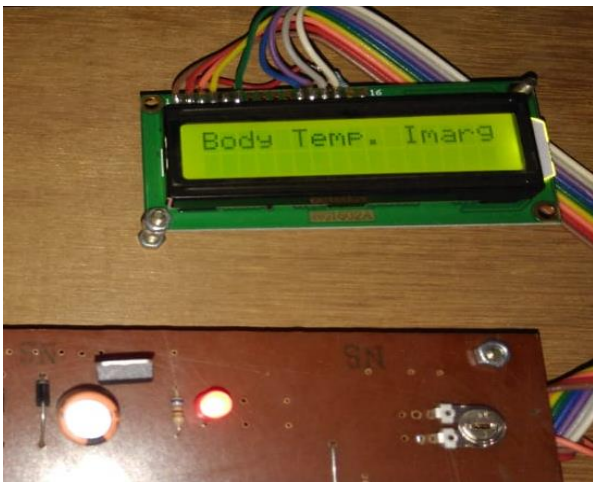
Fig 9. Figure showing Body temp. Emergency on display outside ICU
