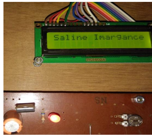
Fig 7. Figure showing Saline emergency on display outside ICU
