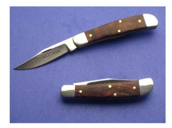
The folder completed by Nathan is a slip joint Trapper style. He choose ATS34 steel for the blade and nickel silver for the bolsters. He choose brass to make the liners out of. The handle material is Desert Ironwood. The closed length of the piece is 3 3/8".
