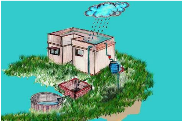
Figure 2: Gutter System of Flat Roof Tops
