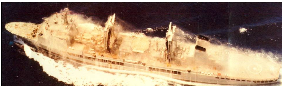
HMAS Success undergoing trials of the Nuclear and Biological wash down system provided by Wormald.
