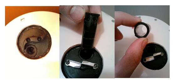
The new epoxy hopper blade is shown above on the left. The old one (center, right) was metal and poorly shaped; it didn't work well.
