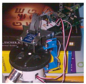
Here is a picture of how the color sensor is mounted. Notice the 3 holes for candy stop in the same place every time. One hole is under the feeding tube, the other hole is under the camera, and the 3<sup>rd</sup> hole is over the chute. The blue bracket holds the IR LED and Phototransistor.
