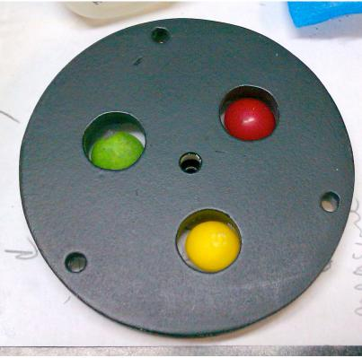
The wheel and interior parts are painted matte black for a reason. It is required to work right. Any other color (or white) will saturate the sensor.
