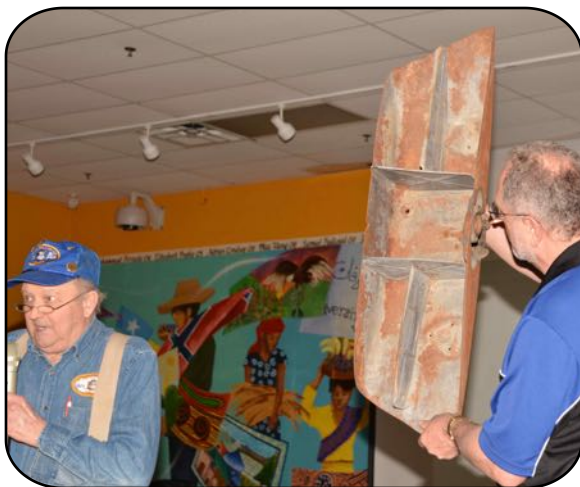
A look inside of how the tank is constructed and where the rust collects.
