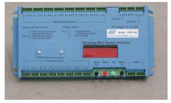
Figure 4: A SDI-12 Interface for connecting 8 vibrating wire sensors to a SDI-12 bus cable.
