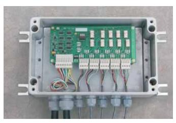
Figure 3: A field mountable Bus Multiplexer in weather proof IP-67 housing shown with its cover removed.
