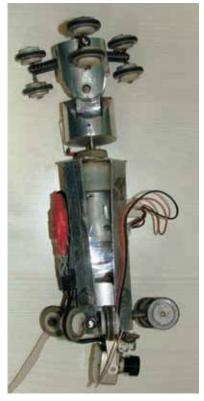
Fig-8: In-pipe robot for internal pipe inspection
