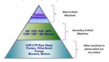
Fig: 1. Pyramid for machinery in power plants
