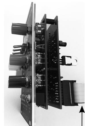
**IMPORTANT: Power connection is red stripe downwards (facing the bottom of the unit) as shown in the picture above. Power diodes on the unit protect against reverse polarity connection.**
