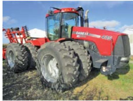
**2008 Case IH Steiger 435:** powershift trans, 435 hp, 12.9 L 6 cyl. diesel, 4 hyd., duals, 720/70R42 tires, GPS 750 Monitor, freshly serviced, 3021 hrs., SN: Z7F108109.
