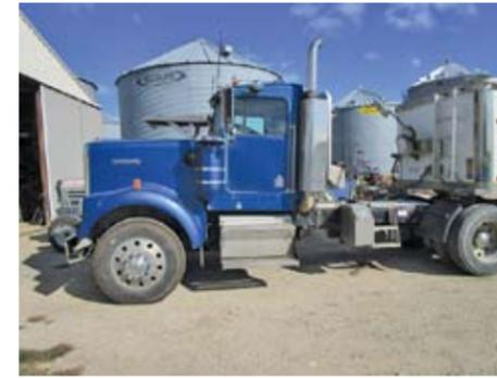
**2004 Kenworth:** W-900 B Model, C15 CAT, single turbo, Eaton 10sp. transmission, dual breathers, dual exhaust stack, 411 rear end, 8 bag air ride, 11R-24.5 near new tires, 650,000 mi., SN: MBN23813
