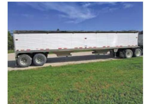
**2009 Timpte Super Hopper Trailer:** 40 ft., Ag hoppers, electric roll tarp, air ride, suspension dump, 11R-24.5 tires, LED lighting, outside aluminum/inside steel SN: H4002 VIN: 9B118951.
