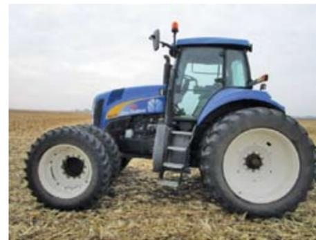
**2009 New Holland T8030:** 299 hp engine, duals, MFWD, powershift, 4 hyd., 480/80R46 rear tire, 380/85R34 front tire, 4500+/- hrs, SN: DFG0045692
