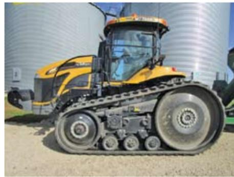
**2012 Challenger MT765D:** 8.4L, 6cyl diesel, 24" rubber tracks, (21) front weights, SISU 265 hp engine, 4 hyd., Pro 700 monitor, 2318+/- hrs., SN: AGCO765CDNCD1246.
