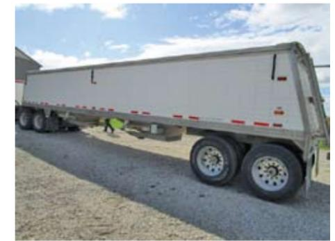
**2013 Timpte American AG Series Trailer:** 42 ft. air ride, aluminum inside/outside, suspension dump, LED lighting, 11R24.5 tires, SN H422, VIN: DB136940.
