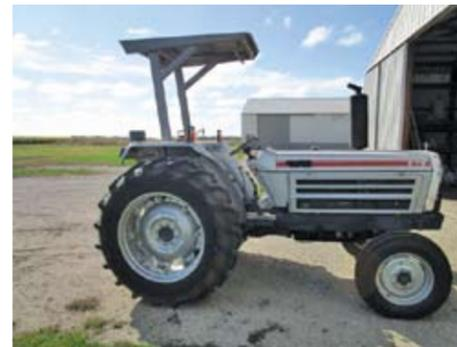
**White-Iseki 2-75:** 5.4L 6 cyl diesel, 2 wd, creeper gears, 540/1000 PTO, 2 hyd, 75 hp PTO, near new tires, 5500+/- hrs.
