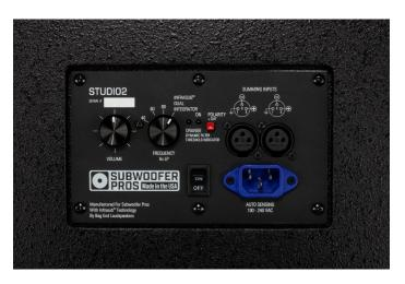
The SUBWOOFER PROS Studio Sub2-18C is a "universal" sub used for bass extension of any studio monitor. It is sealed and self-powered, offering bass extension to 16Hz. It has a compact cabinet using an 18" high excursion sub driver with an easy to use control set. It has built in Left/Right XLR summing inputs and a low pass filter at 4 different frequencies of 95Hz, 80Hz, 60Hz, and 40Hz. The different low pass frequencies make it adaptable to various size "main" speakers.
