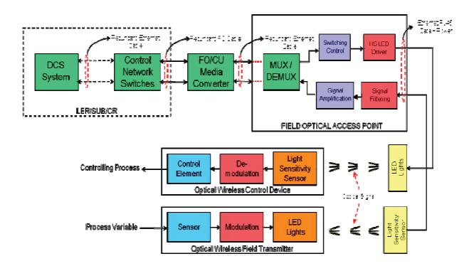
Figure.2: Block diagram of Li-Fi instrument communication network.
