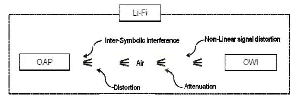
Figure.8: Signal flow in Li-Fi instrument communication.
