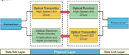
Figure.1: Basic block diagram of full duplex of Transceiver System.
