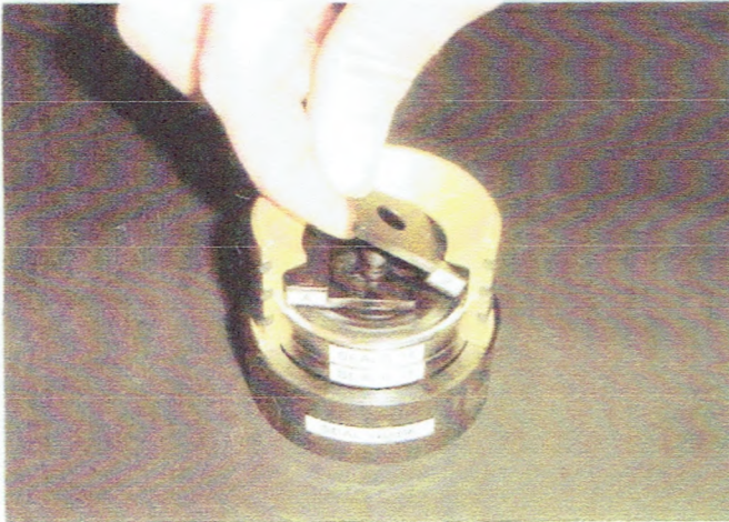
Step 3 Place Jaw B in cavity over screw.
