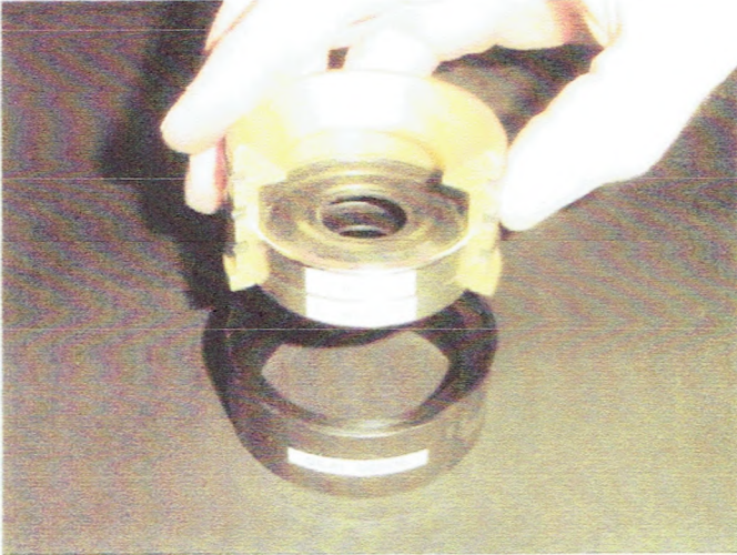
Step 1 Place axle seal housing into counterbore of seal guide.
