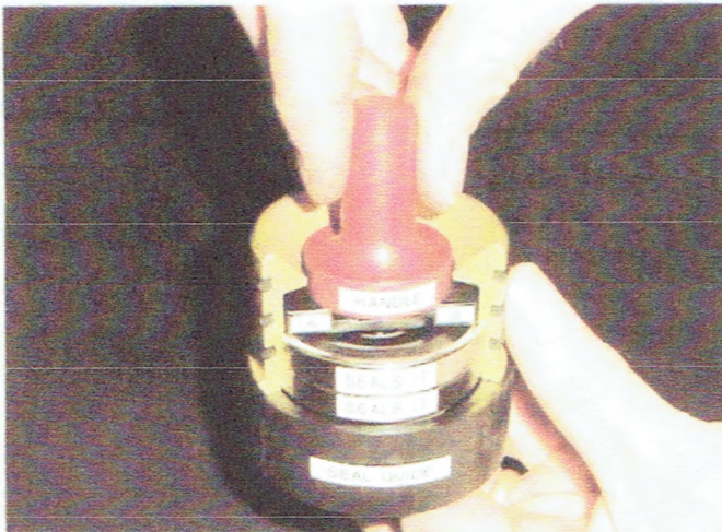
Step 5 Assembly ready for arbor press.
