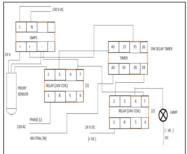
Fig.4. Connection Diagram
