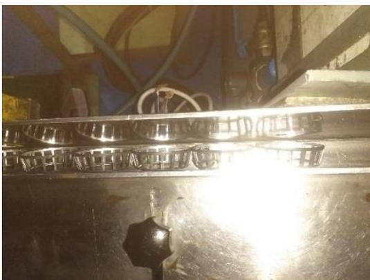
Fig .1 Bearings are stuck in Channel
