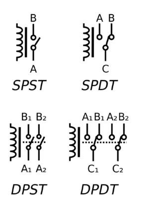
Schematic symbols of relays of an electrical system of which you are!
