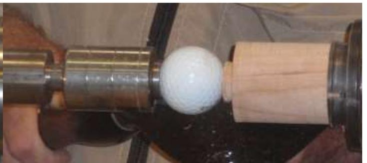
Here Steve has turned the bottom of the box around so that he can remove the tenon
