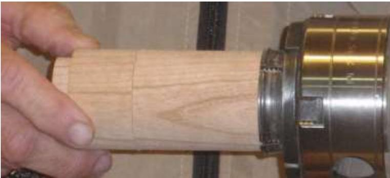
The box is mounted so that the bottom can be hollowed.
