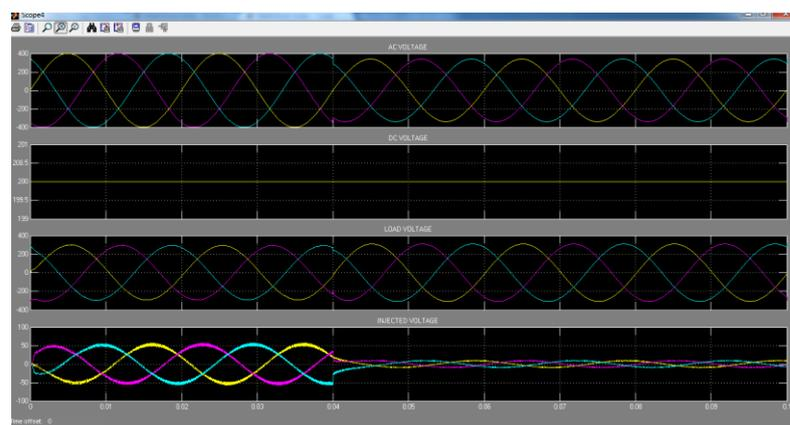
Fig. 9. Simulation Result for Voltage Swell and DVR Compensation
