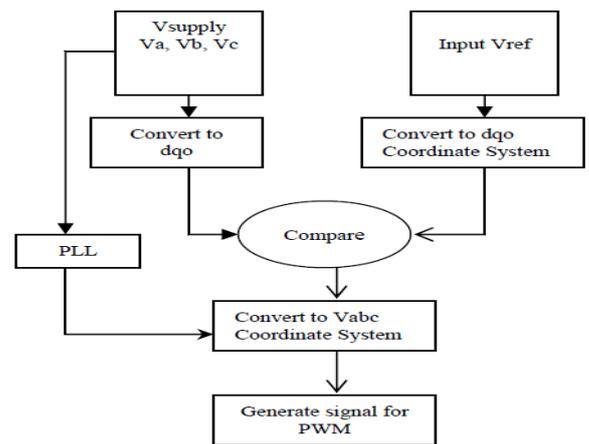
Fig. 3. Flow chart of feed forward control technique for DVR based on dqo transformation
