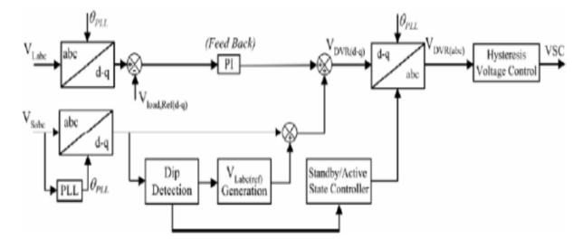
Fig. 5. Control Structure of DVR
