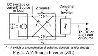
For simplicity of steady state analysis, inductors and capacitors are assumed to be ideal and are considered to have equal values. The inverter's action is replaced with a current source plus a single switch.
