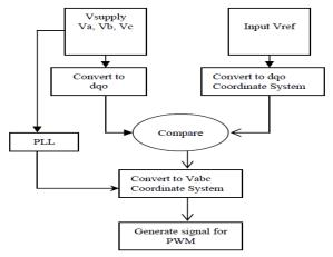
Fig. 3. Flow chart of feed forward control technique for DVR based on dqo transformation
