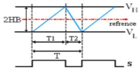
Fig. 4. Hysterisis Band Voltage Control  $T_1 + T_2 = T_c = 1/f_c$
