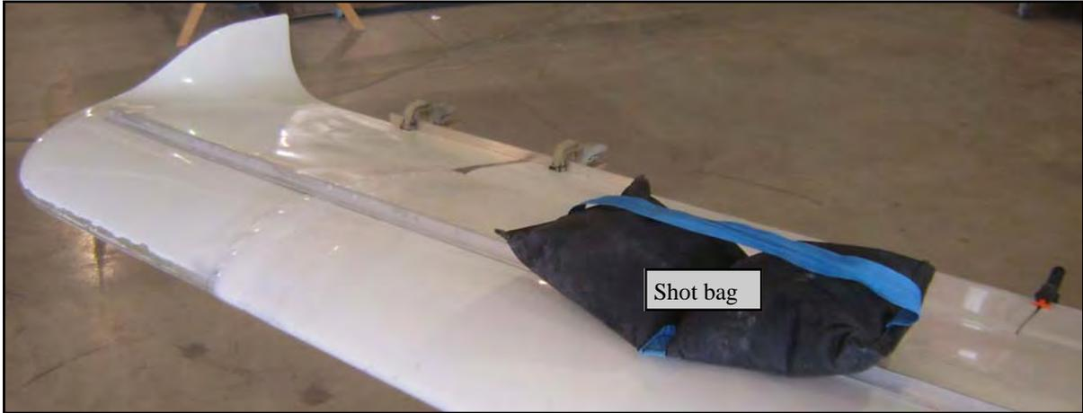
9. Slide the wing tip in place and clamp the trailing edge to the angle aluminum.
