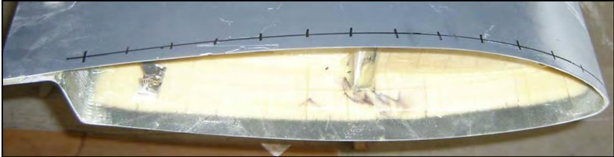
8. Use the photo below as a reference for setting up some items that will help fitting the wing tip. Items need are: 2 foot piece of scrap angle aluminum. At least a 4 foot piece of scrap angle aluminum, weighted bag (shot works), clamps and clecos.
