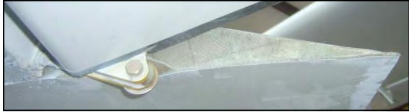
31. Remove the tip and glue in the close out rib with epoxy and floc. Remember to sand up the inside of the wing tip for a good bonding key and pre wet both surfaces with epoxy before putting the floc mixture in place.
