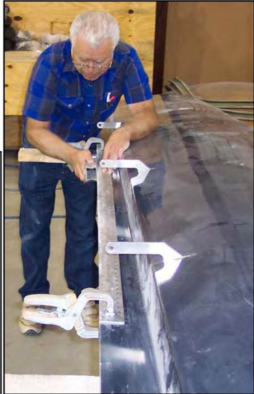
**Note:** It is easiest to fit the wing tips if sections 12 and 13 have been completed. This will provide the best fit and alignment of either set of wing tips.
