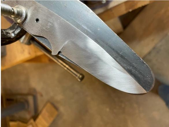
The final grit I hand sand to will be 800 and that will be lengthwise in the same direction as the initial 220 grit. When the only scratches showing on the blade are 800 grit switch to a new section of paper and make long smooth strokes to try and avoid the j-hooks from stopping and changing directions.
