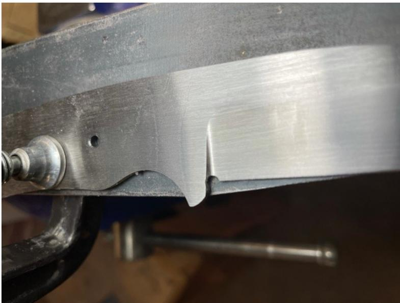
Once there are no belt scratches in the plunge area I switch back to the first stick and sand diagonally with 400 grit until I cannot see any of the 220 lengthwise scratches. Then I sand with 600 grit diagonally in the other direction until there are none of the 400 scratches showing.
