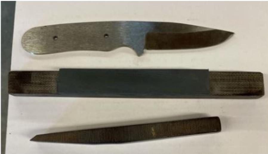
Both are made from micarta and the black or grey pad is poundo board from Tandy that is glued on. The main tool is approx. 9" long and  $\frac{3}{4}$ " wide. The other one is for getting in the plunge area (more on the later).
