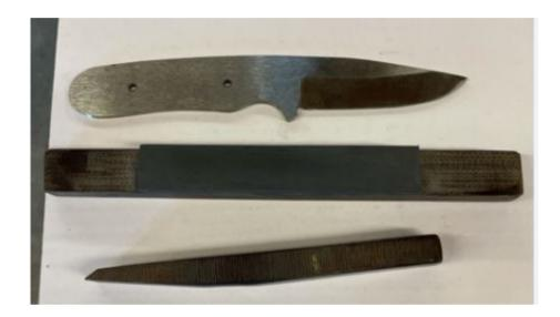
Both are made from micarta and the black or grey pad is poundo board from Tandy that is glued on. The main tool is approx. 9" long and ¾" wide. The other one is for getting in the plunge area (more on the later).
