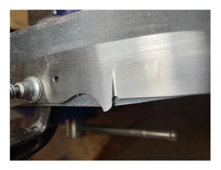
Once there are no belt scratches in the plunge area I switch back to the first stick and sand diagonally with 400 grit until I cannot see any of the 220 lengthwise scratches. Then I sand with 600 grit diagonally in the other direction until there are none of the 400 scratches showing.
