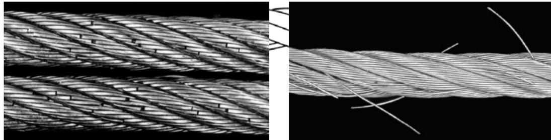
*Excessive wear of wires*
