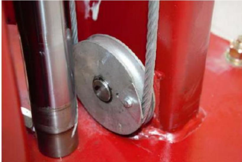
**Figure 22: Lower Pulley install**
