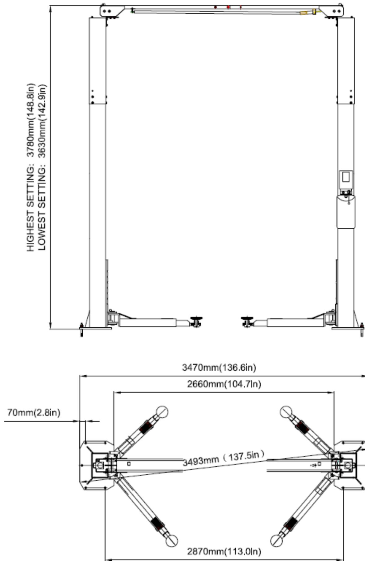
***Deduct 150mm/5.9 in. from the width dimensions for the narrow installation***
