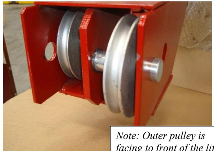
*Note: Outer pulley is facing to front of the lift*
