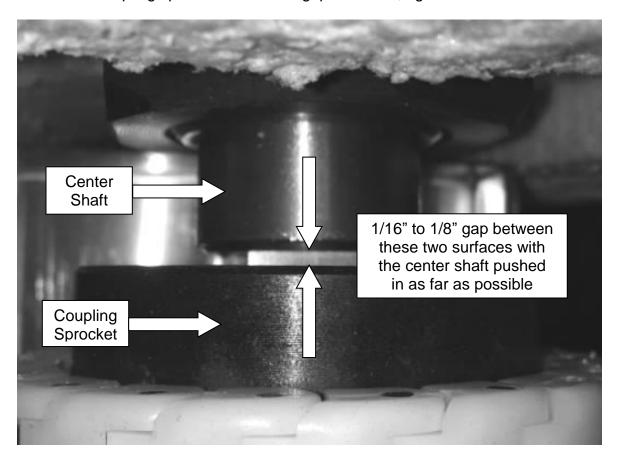
6) With the installation now complete, clean and grease the o-ring area of the center shaft prior to final assembly.
