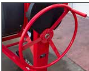
Oversized drum wheel makes discharge of material easier.
