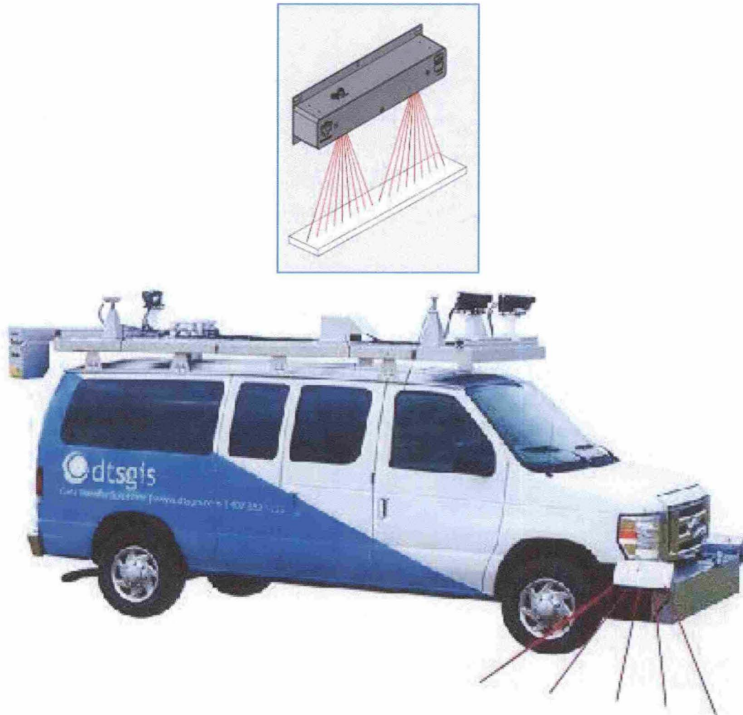
Figure 1 - Laser Profiler and Van Survey Equipment
