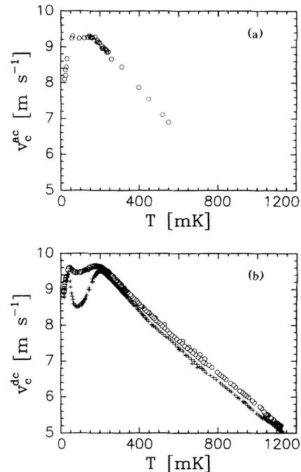
FIG. 1. (a) Critical velocity for single phase slips during oscillatory flow as a function of temperature. (b) Critical velocity for dc flow in two different directions (at an applied pressure of  $\Delta P \approx 0.5$  Pa) as a function of temperature. Circles represent  $v_c^{\text{dc}+}$  and crosses  $v_c^{\text{dc}-}$ .
