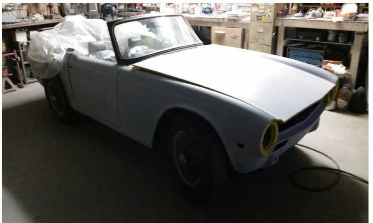
Exterior in primer (overspray from interior repair)
