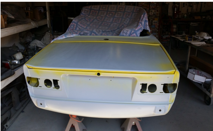
Rear deck in primer (note overspray from boot repair)
