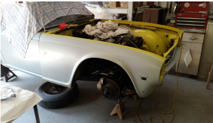
Engine bay paint prep (above)
