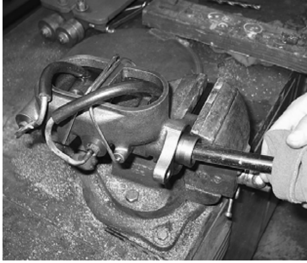
Using his handy-dandy bleeding lines, IJ bench-bled the master cylinder.
