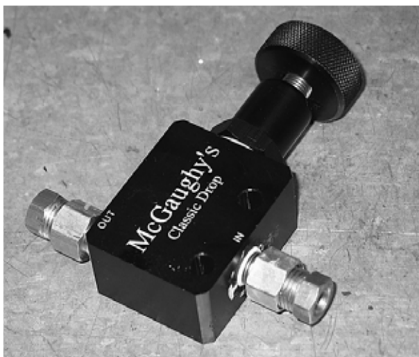
The last item to be installed was the McGaughy's adjustable proportioning valve.
