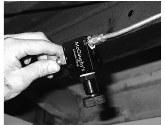
IJ picked a spot along the frame, and then cut and double-flared each end of the line. At this point we could bleed all four lines.
