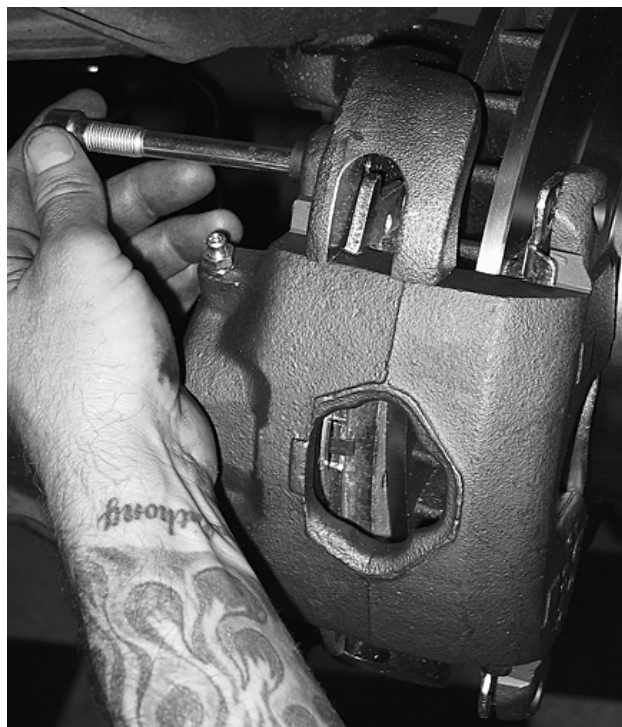
...which were then fit over the rotors and bolted to the spindles.
