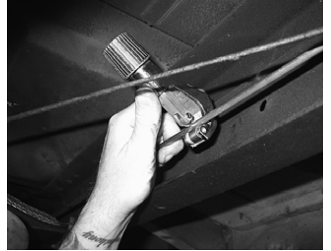
The prop valve can be located anywhere along the rear line between the distribution block and the "T" are the rear.
