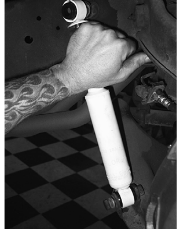
Next, IJ installed the new shock in the stock location.
