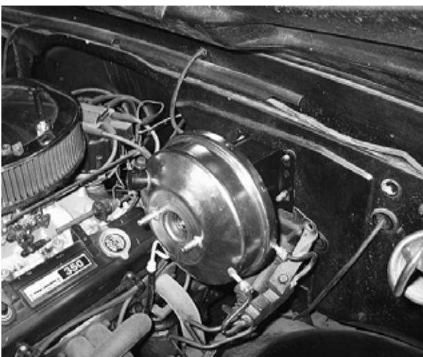
The 9-inch booster and pushrod were installed onto the stock studs on the firewall and secured.
