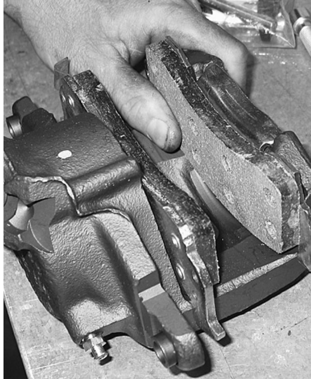
New, semi-metallic pads were fit into the calipers...
