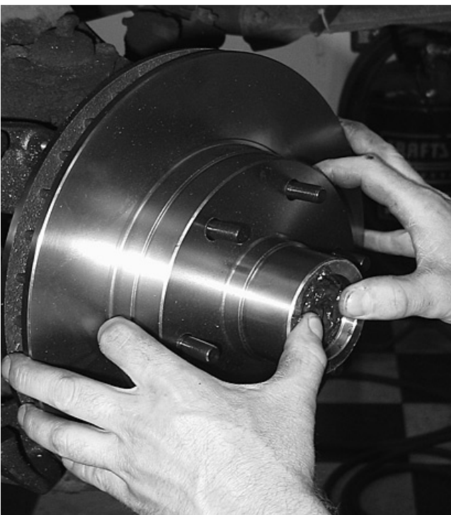
At this point, the rotor, along with the outer bearing, were installed onto the spindle.
