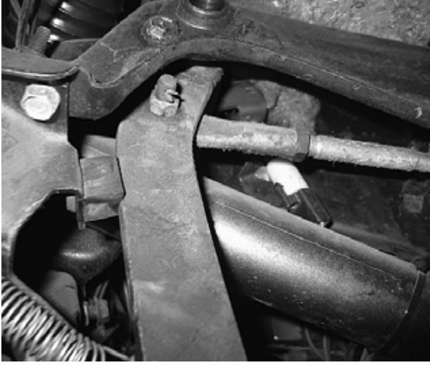
Under the dash, IJ removed the pushrod from the brake pedal.
