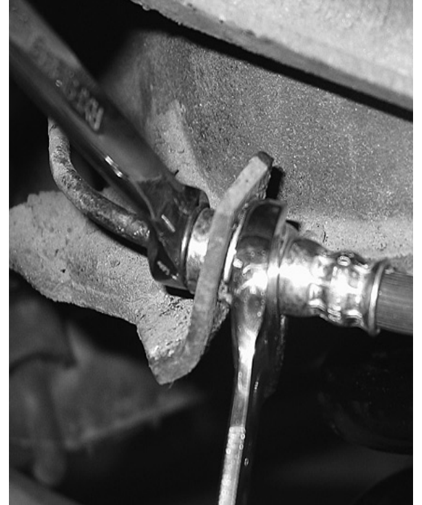
The new brake hose was then attached to the factory hard line.
