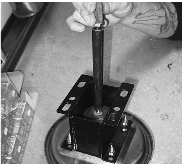
IJ installed the stock rod end onto the new pushrod.
