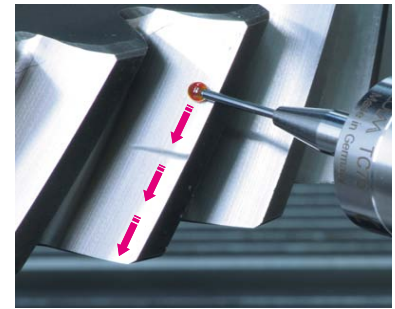
Scanning procedure for checking of workpiece surface
