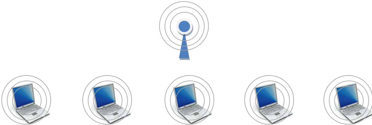
Figure 2: General setup of a wireless network, illustrating that both the AP and the end devices emit RF EMFs.
