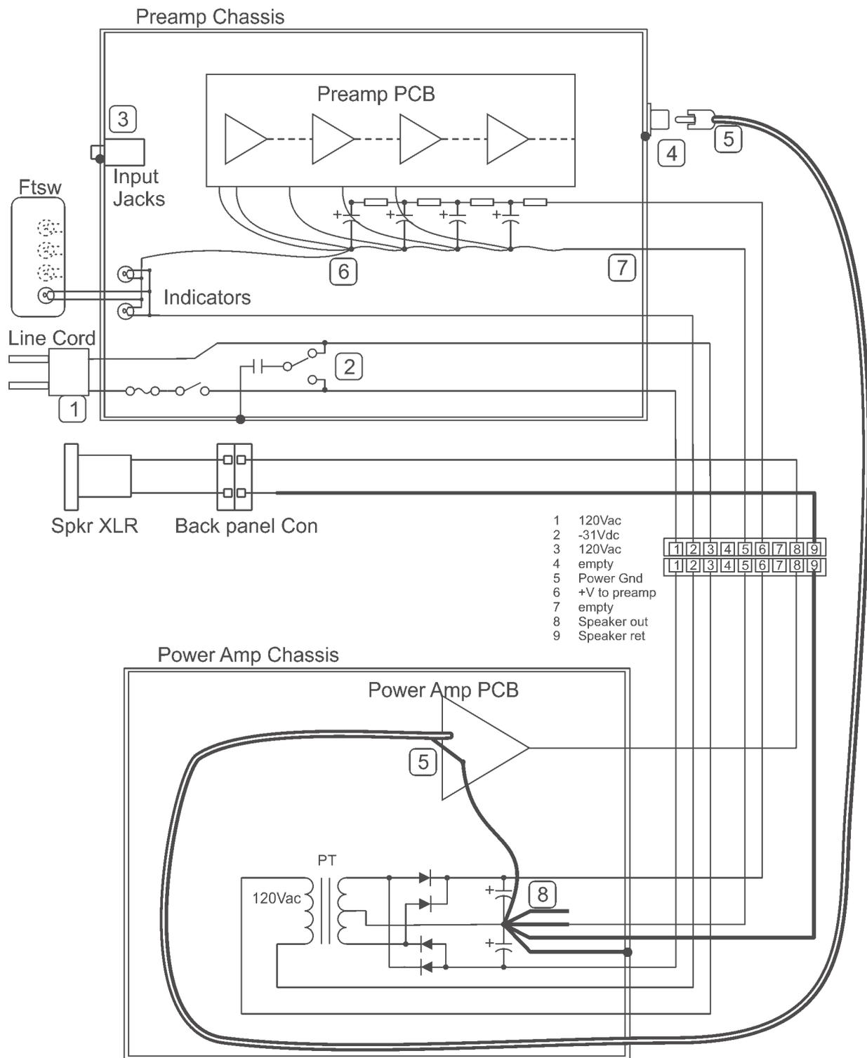
However, there is no connection from the power supply ground for the preamp circuits [7] to the metal shell of the preamp at all. Instead, the preamp power ground is carried on one wire of the cable to the
