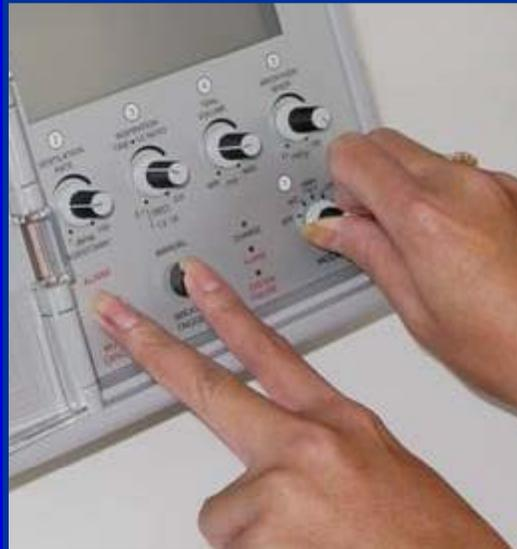
**To enter the USER PROGRAMS Menu, simultaneously press the MUTE and MANUAL BREATH/TRIGGER Pushbutton Switches while turning the MODE Control Switch to A/C, SIMV, CPAP, or CAL.**
