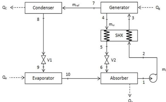
Hence to utilize the exhaust gases and waste heat from an engine the vapor absorption refrigerant system can be put into practice, which decreases the cooling water temperature. That leads to proper cooling of diesel engines walls there by increases the overall performance of diesel engine and also reduce the problem of leaking of cooling water which is caused by the over heating of engine parts.
