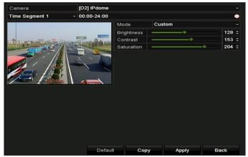
Figure 15-6 Image Settings Interface (IP Camera)
