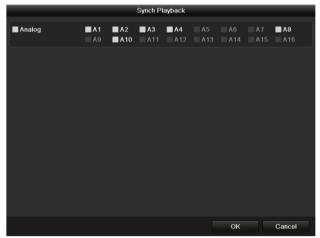
Figure 6-7 Select Channels for Synchronous Playback
