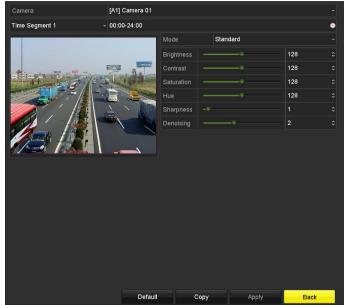
Figure 15-5 Image Settings Interface (Analog Camera)
