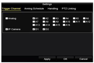
Figure 9-15 Set Trigger Cameras of POS
