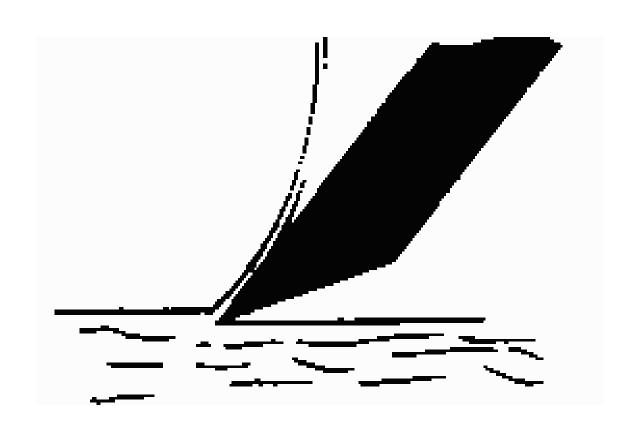
The common belief of the twist on a drill bit is for chip removal, which it does do, BUT the twist gives the cutting edge a positive angle which helps PULL the drill bit into the work piece
