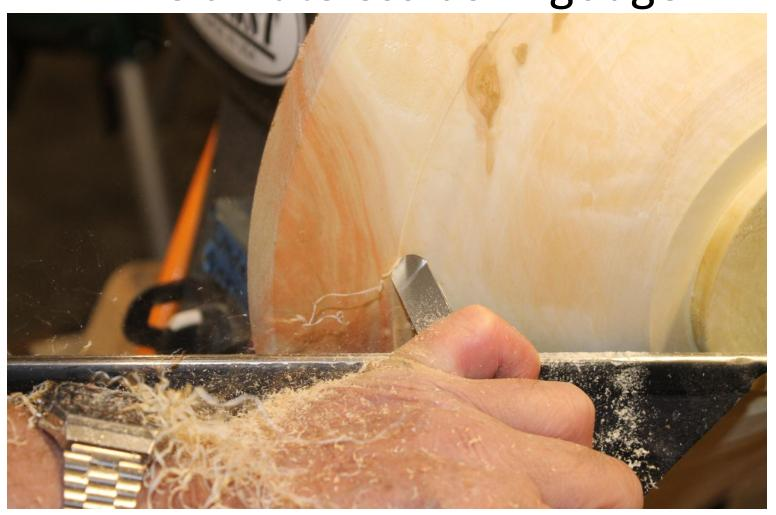
By using the cutting edge almost parallel with the rotation of the lathe, The finish is smooth.
