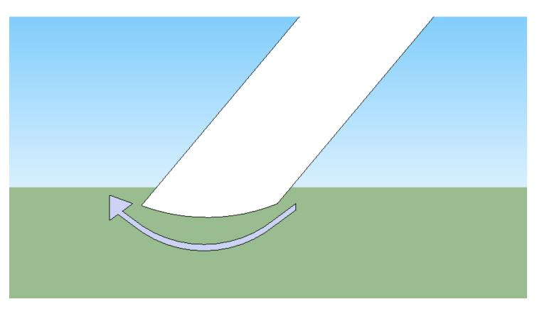
(Exaggerated hollow grind bevel)
