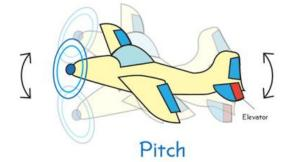
Use the elevators to control Pitch
