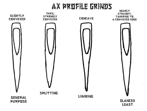
When sharpening your axe be mindful of the bevel or angle at the bit end. An axe is not a straight consistent wedge. The angle of thickness is different as you move up the axe bit. Most axes have a 30°-40° degree angle at the end of the bit and a 15° -20° degree angle about 1/2" from the cutting edge. The bulge away from the end of the bit is what provides the axe its splitting power.
