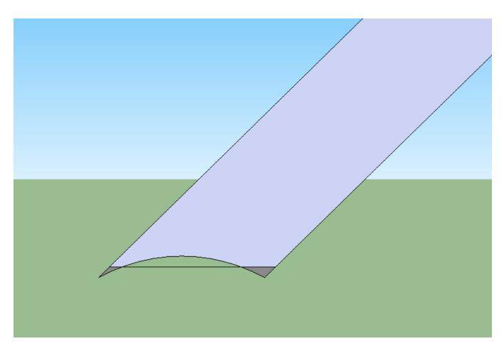
Notice that honing changes the cutting action. Instead of digging in, it will move straight ahead. It is still sharp, it just cuts (feels) different.
