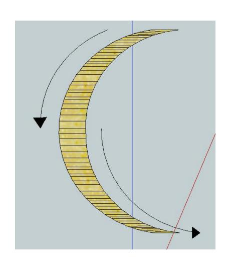
I use the gouge with the flute about half open to rough turn. It may be hard to see, but I am rubbing the bevel to control the depth of the cut. Shear Cut.
