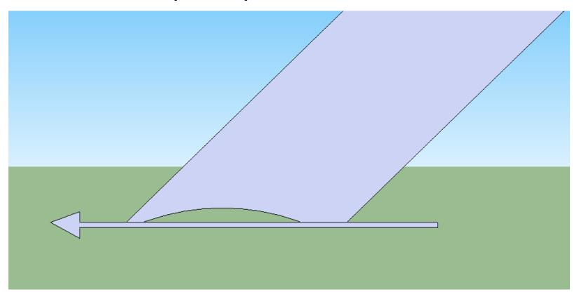
Much less used is a convex grind bevel, but it has an advantage; it works like a carving chisel. It wants to move up and out of a cut.
