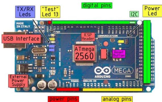
Fig 2: Arduino prototype Development Board
