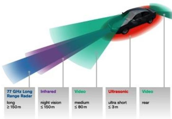
Fig 1 : Range of different sensors
