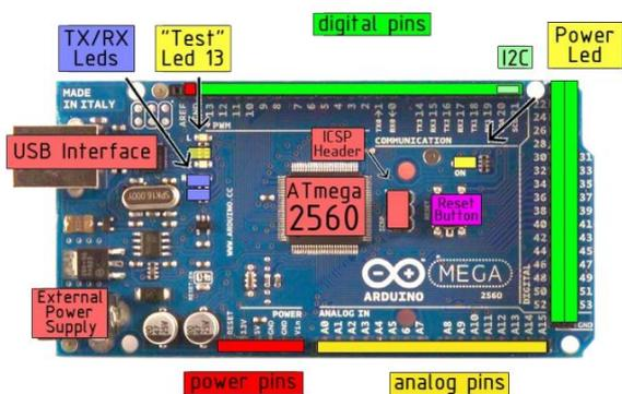
Fig 2: Arduino prototype Development Board
