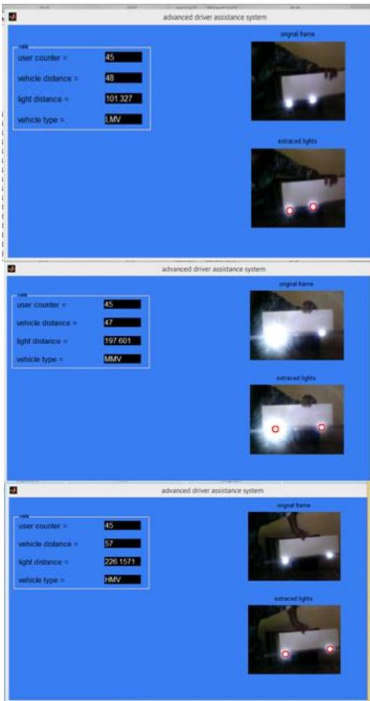
Fig 11: Developed GUI showing user counter, vehicle distance, light distance (a) LMV (b) MMV (c) HMV
