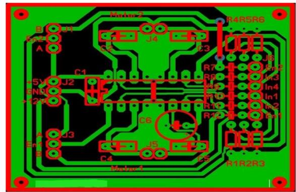
Fig 5: Final Printed Circuit Board
