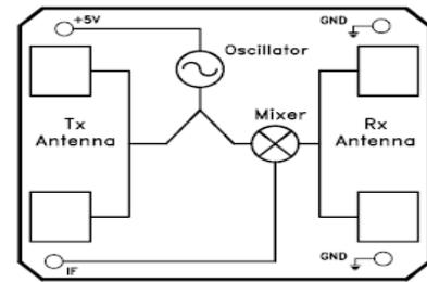
Fig 3: Block diagram of Radar Module
