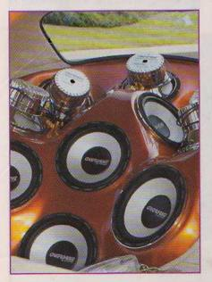
LEFT, custom-molded fiberglass rear enclosure holds eleven Blaupunkt 10-inch Overdrive speakers. BELOW, custom bodywork includes Dodge Neon door handles, and hidden hinges, from the Rocky Hinge Company, for a clean look.
