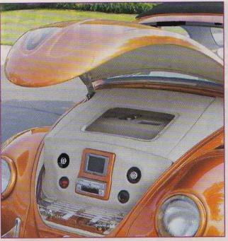
LEFT, one of the highlights of this car is a Blaupunkt electronics, like in the trunk where there is a custom enclosure housing a modified gas tank, two Stinger dry cell batteries, Ron Francis fuse block, master power switch, front-mounted TV and DVD player, 3speakers, Street Glow neon and strobe lights, and more. BELOW, interior is just as deckedout with Blaupunkt electronics, including changer, navigational unit, dual five-inch Gauges are trick Cyberdyne digital.
