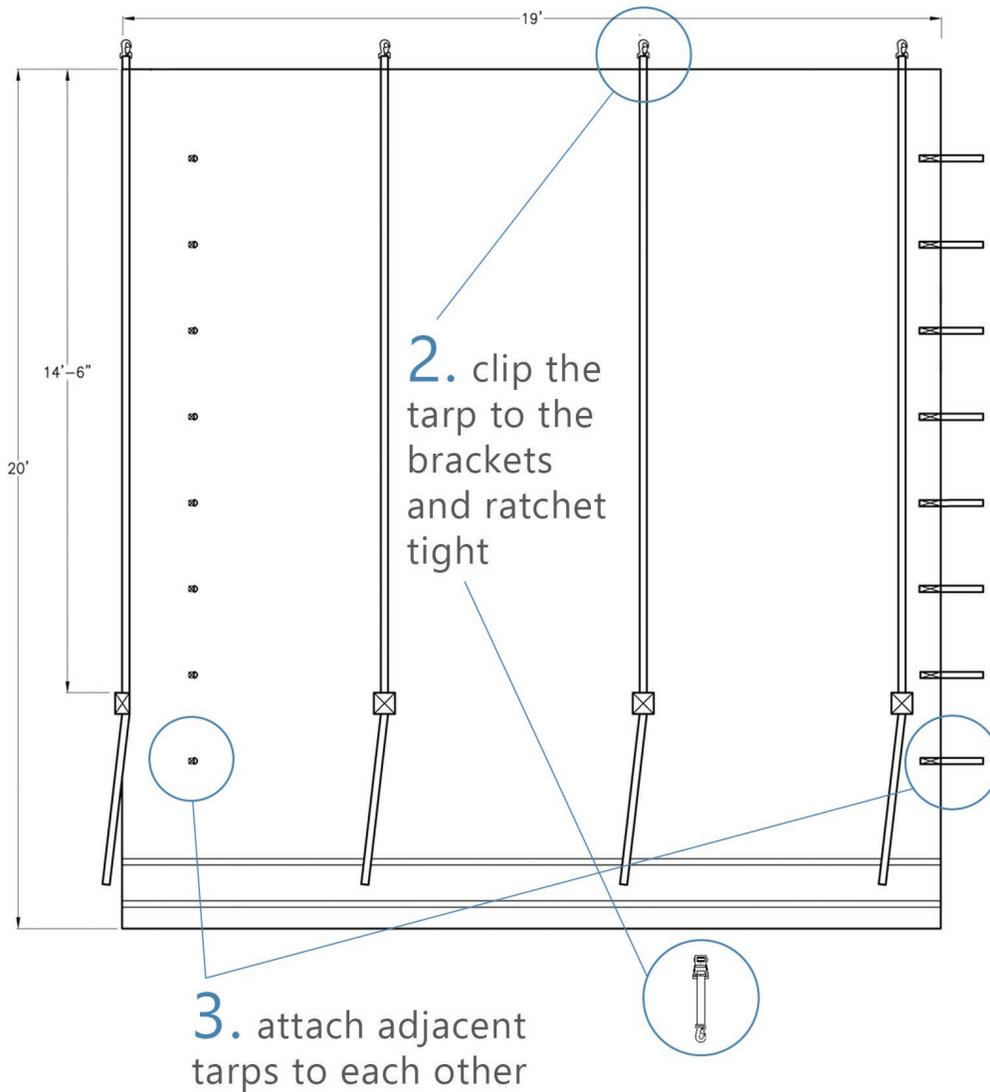
1. anchor the steel plates to the floor slab
