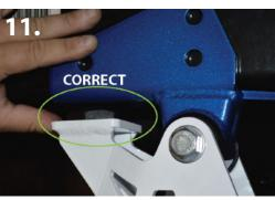
14. With the brackets fully assembled, lift the frame mount up and place against the bottom of the frame. Making sure there is no gap between the bump stop and the frame mount. (pic 10-11)
