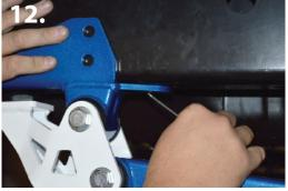
15. Mark the hole on bottom of frame. (pic 12)
