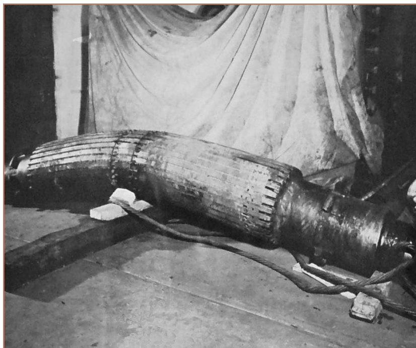
figure 5. Bent rotor from the Böhlen power station near Leipzig that was destroyed by an Operation Outward balloon on 12 July 1942 (from The National Archives of the United Kingdom, folder #ADM 199–848).
