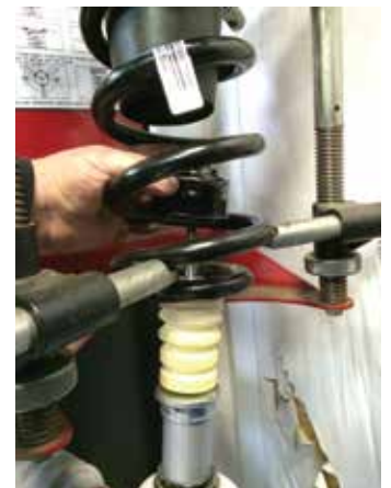
Installing the factory spring & Inner bump stop cup to the new McGaughy's strut.
