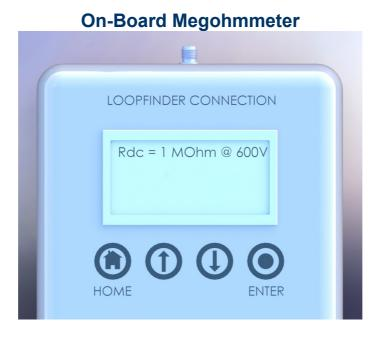
Measure the high voltage leakage resistance of the loop to ground
