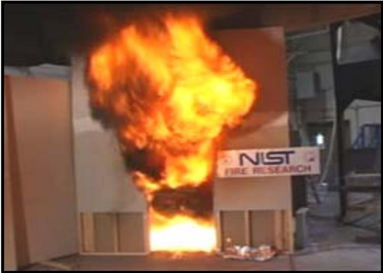
Figure 3 – Flashover and subsequent Backdraft
