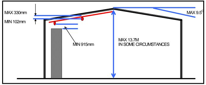
Figure 10 – Basic ESFR dimension constraints
