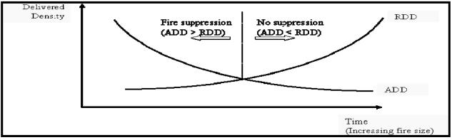
Figure 3 – Sprinkler Suppression Concept
