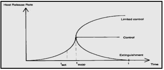
Figure 2 – Sprinkler Control and Suppression
