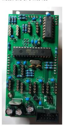
Install the seven MCP602 op-amps into the remaining sockets
