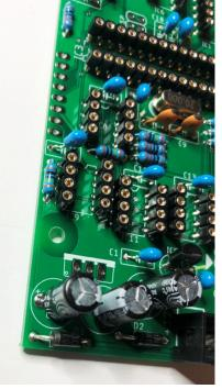
Install and solder the 7805 voltage regulator IC4
