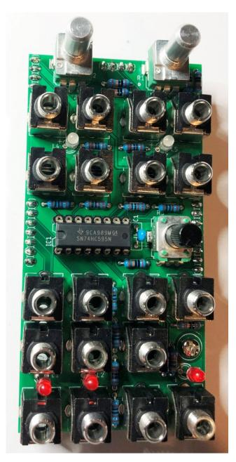
Carefully slide the panel over all of the seated components.
