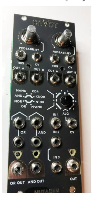
Flip the board over and solder one pin of each jack and potentiometer to hold it into place. If you bent the LED pins to sit it against the desk, bend them straight again. Direct the LEDs into their holes and push them in firmly. Turn the board on its side and inspect the LEDs are seated correctly and that everything is seated nicely. When you are happy that everything is seated well, solder the rest of the remaining jack, pots and LEDs.
