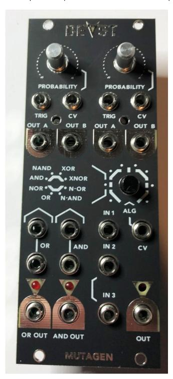
Install a few of the knurled nuts (I did 6) firmly and install washers and nuts onto the two bushed potentiometers – FINGER TIGHTEN only otherwise if you overtighten the potentiometers will lift off the PCBS and/or twist. This was enough tension to allow me to flip the board over to solder everything without it falling apart. Carefully test it out – you may need to install knurled nuts onto more jacks to get more tension.
