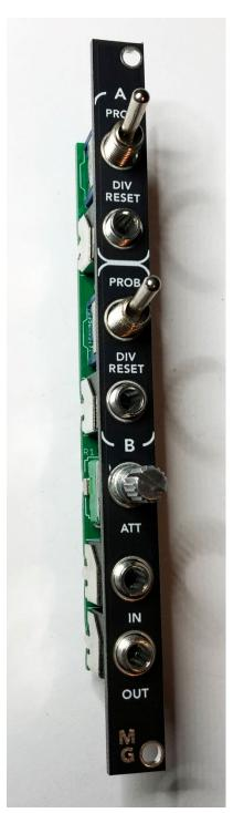
Install the knurled jack nuts, switch nuts and tighten. Place a nut on the potentiometer and finger tighten until firm and the nut is aligned perfectly with the side of the panel. The potentiometer may rise slightly from the board (less than 1mm) but this is okay so that the nut is aligned and not jutting out over the side of the panel.
