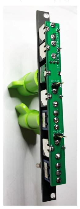
Flip over and install the knob onto the potentiometer. Refer to the user guide for instructions on how to connect the expander to Mutagen.
