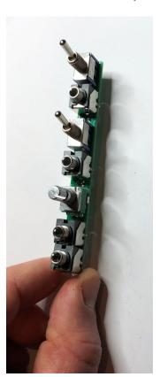
Carefully slide the panel over the switches and jacks
